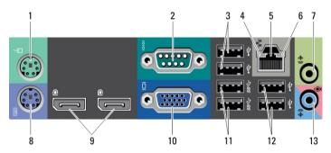
Figure 4. Back Panel View of Small Form Factor
